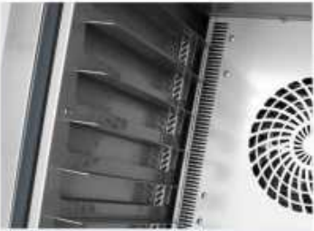
Container Rack Suitable container size: 530x325mm and 600x400mm
