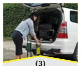
**EASILY ADJUSTED** She then lowers the platform supports into a folding position by simply flipping a latch on each side and sliding the supports in a downward position.
