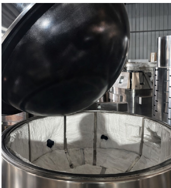
Stainless steel cooking bowl with hinged cover, designed for direct gas heating and high-temperature food processing.
