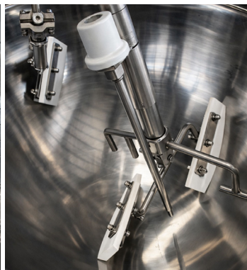
Planetary mixing assembly with fixed shaft and PTFE scrapers, ensuring uniform agitation and wall-scraping during cooking.
